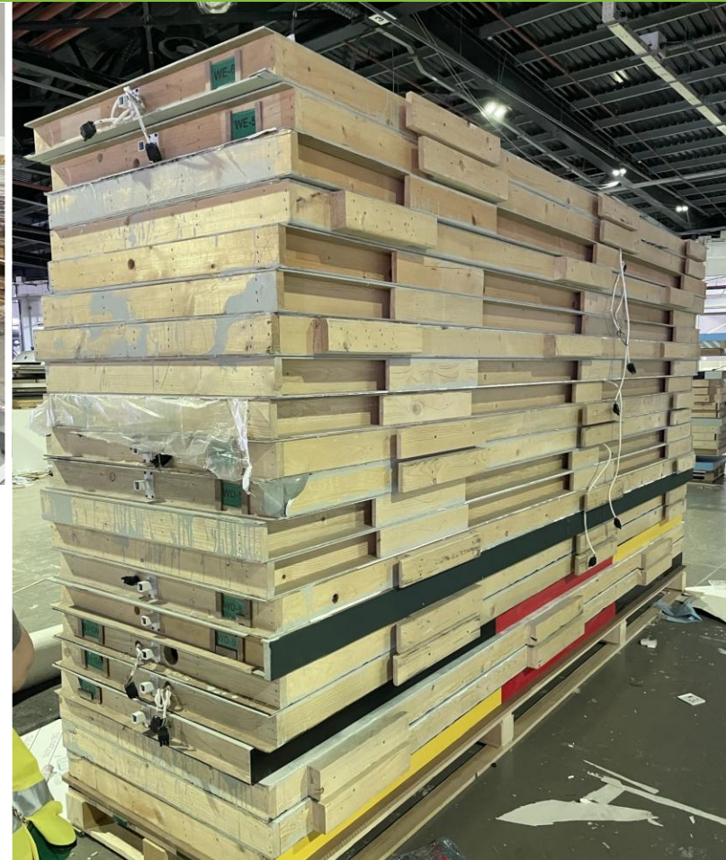
Stock panels with sheets and wooden grooves to lock in down the side
