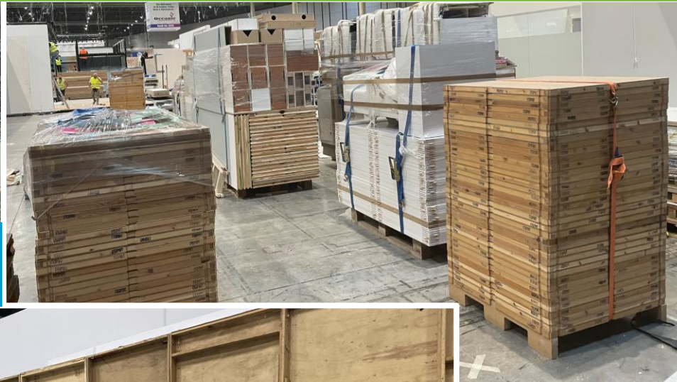
Stock panels with sheets on both sides and access ports for fixings
