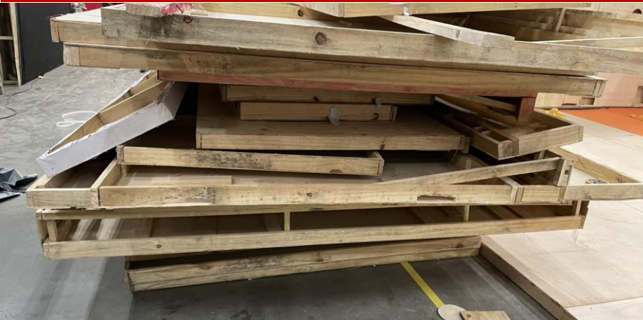
Inconsiderate stacking on pallets or trucks
