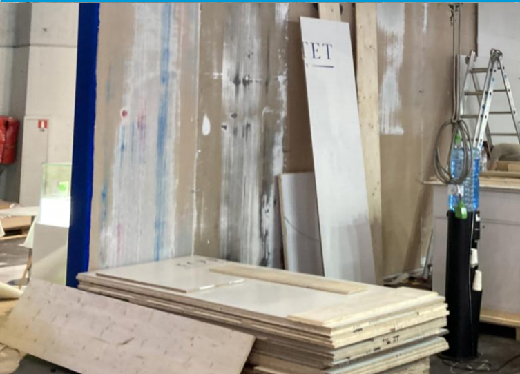
Evidence of reused painted panels or stock panels
